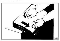
When paper edges stick together or paper is not fed to the machine, shuffle the paper as shown.
